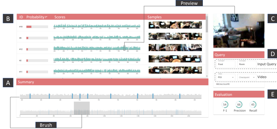
Figure 5.4: Prototype Overview. A: Summary View presents two temporal bar charts, which shows the overall scores and the summarized shots. The bottom bar chart shows the overview of all the shots, while the top bar chart zooms into the detail decided by the brush in the bottom chart. B: Intent View list all the basis intents with their probability, shot scores, and representative samples. The samples are selected with the highest score. C: Preview View plays a GIF of the user-hovering shot. In this case, the user hovers on the highlighted shot in intent #12, which includes a room scenario. D: Query View allows the user to change the query and makes the model rerun. E Evaluation View shows the quantitative result of the summary.
