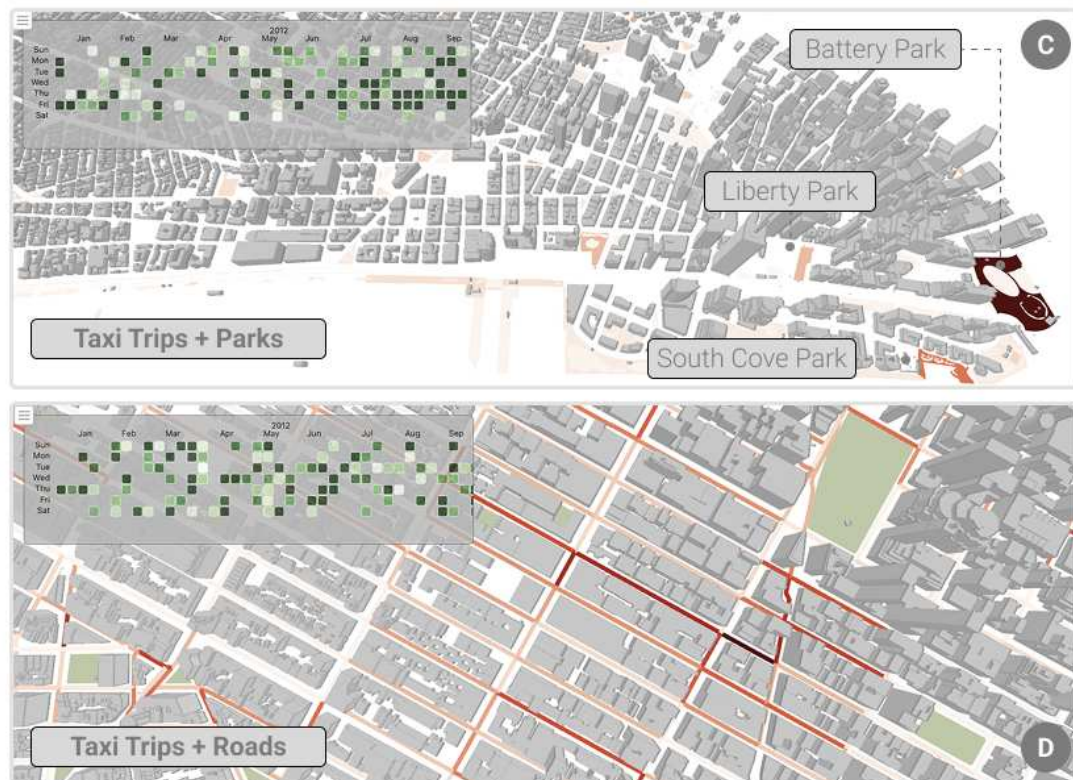
Figure 6.1: Usage scenario of PyAutark. In a few lines of code, users can explore urban spatiotemporal datasets supported by city infrastructure data. A and B show the code needed to generate the interactive spatiotemporal visualization provided by PyAutark. C shows the distribution of taxi pickups around parks in lower Manhattan. D shows taxi trip data projected onto Manhattan’s road network.
