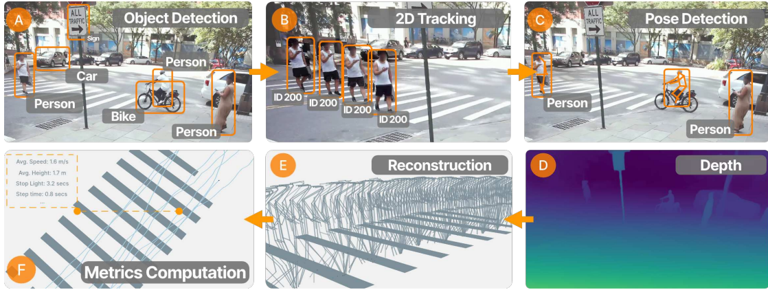
Figure 4.1: Crossroads’s Data Processing Pipeline, broken down into six steps: Operations in 2D include Object Detection (A), 2D Tracking (B), and Pose Detection (C). Once these operations are done, the pipeline proceeds to operations in 3D space. First, depth computation is computed for each video frame (D). With that information, we can then reconstruct different actors (such as pedestrians and cyclists) in the 3D urban space (E). Finally, once the urban space and actors are reconstructed and tracked in 3D, we automatically compute and display different metrics, such as average speed and time taken between steps (F).
