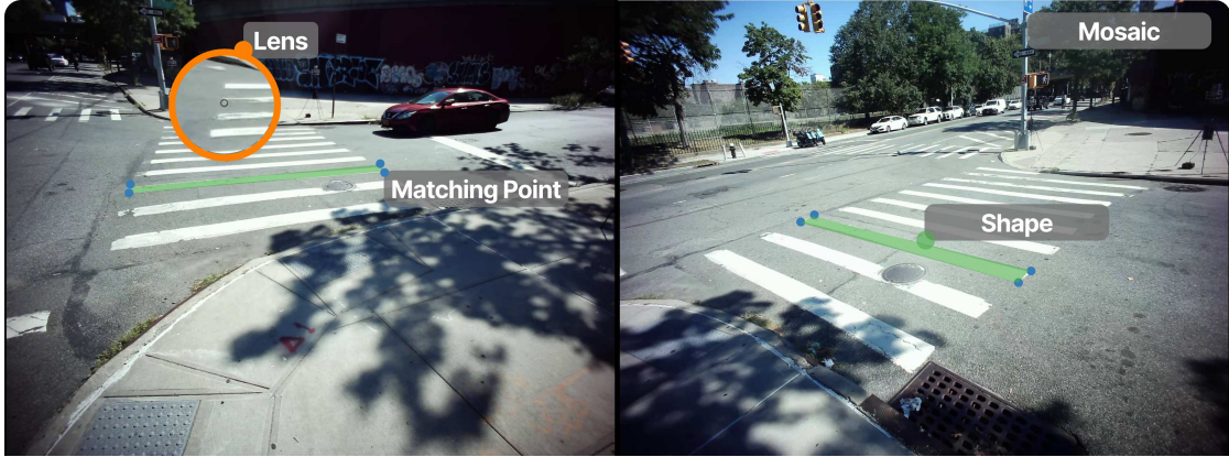
Figure 4.4: Mosaic of frames employed to define matching points from different cameras used in the registration process. To increase the user precision, the system implements a lens-inspired tool.
