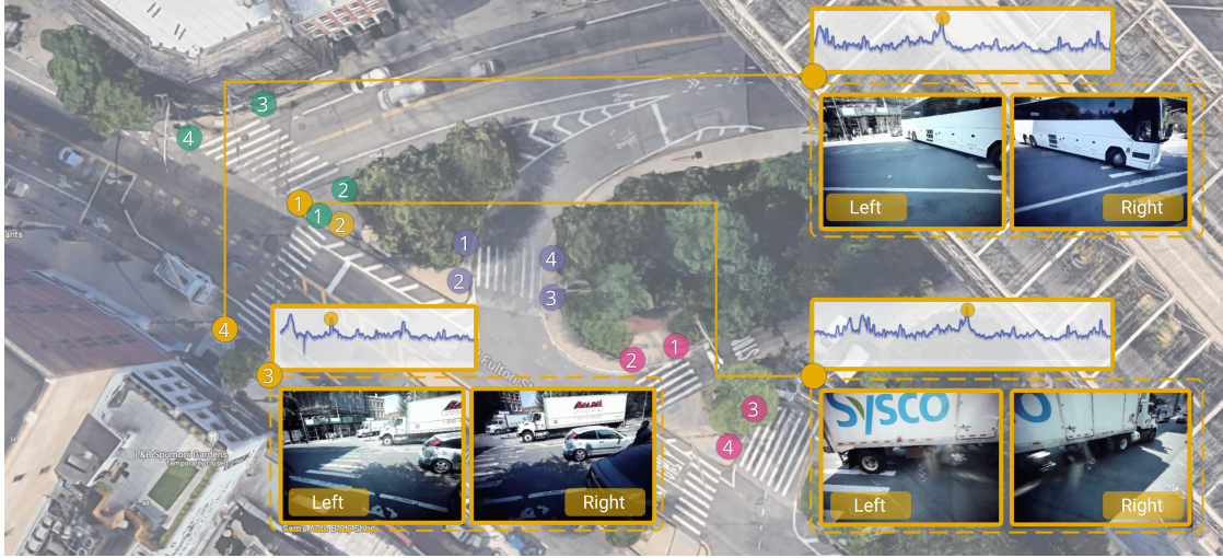
Figure 3.12: Sensor positions during data acquisition at DUMBO, Brooklyn. Colors indicate recording sessions, and numbers denote the sensor. Above each synchronized video frame, we highlight the relative data point in the audio time series (in decibels). It can be shown that events that can be seen in the video, such as the passing of a bus, have a corresponding peak in the audio data.
