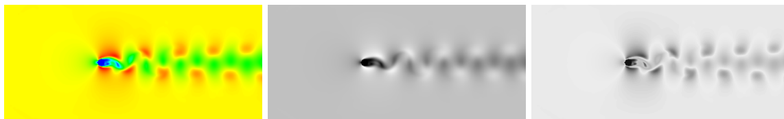
Figure 6.3. Velocity magnitude. Rainbow (left) and gray scale (middle) color maps were applied to a 2D flow simulation using a spectral element code for solving the incompressible Navier-Stokes Equations. Note how red regions on the rainbow color map are over-emphasized while green regions “blur” details that are shown in the gray color map. The image on the right is the decolorized rainbow color map.
