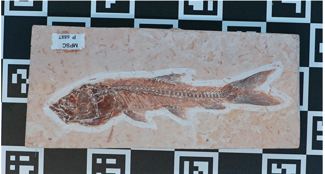
Figure A.1: An example image of the real fossil object. A ChArUco Board is placed underneath the fossil as background.
