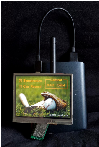
Figure 6.11: Portable orchestrator radio based on nRF24L01P+ 2.4 GHz radio module with touch screen booster pack of Tiva C microcontroller as the input device.
