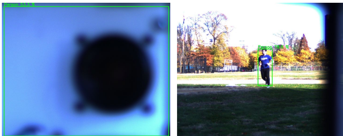
Figure 6.13: Video samples with object detection overlay acquired using the second prototype. Of notice is the camera's self-identification as a person and poor dynamic range in presence of sun shadows, which negatively impact the real-time tracking.
