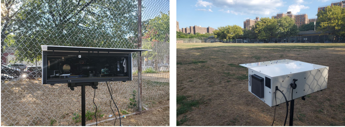
Figure 6.18: Third LegoTracker prototype with improved performance (Full HD recording at 150 fps). The photos were taken during in-field testing.
