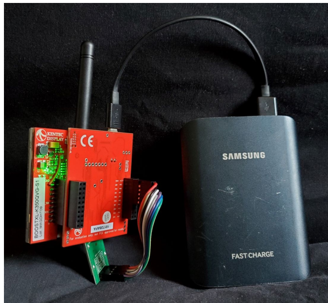
Figure 6.11: Portable orchestrator radio based on nRF24L01P+ 2.4 GHz radio module with touch screen booster pack of Tiva C microcontroller as the input device.
